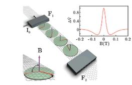
... precession of spin-polarized charge current gives rise to quantifiable dephasing by means of non-local voltage measurements.
